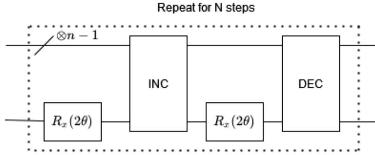
**Figure 32:** General circuit for Staggered Quantum Walk
