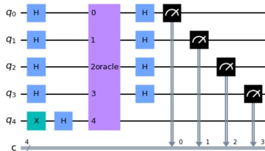
Figure 45: DJ circuit for n=4 qubits
