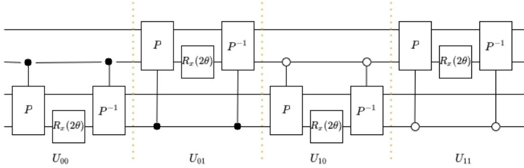
**Figure 38:** 2D SQW evolution operator circuit for one walk step on a lattice with 16 vertices using 4 qubits
