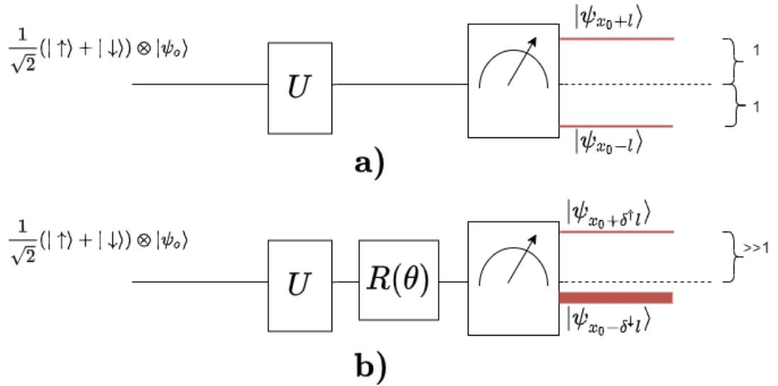
**Figure 22: a)** The particle enters the conditional displacement box  $U$  after being localised in point  $x_0$ . It is displaced up or down by  $l$  based on its spin degree of freedom. When it exits its spin is measured in the  $z$  basis. ( $M_Z$ ). With probability  $\frac{1}{2}$  it is found displaced by  $l$  resp.  $-l$ .
