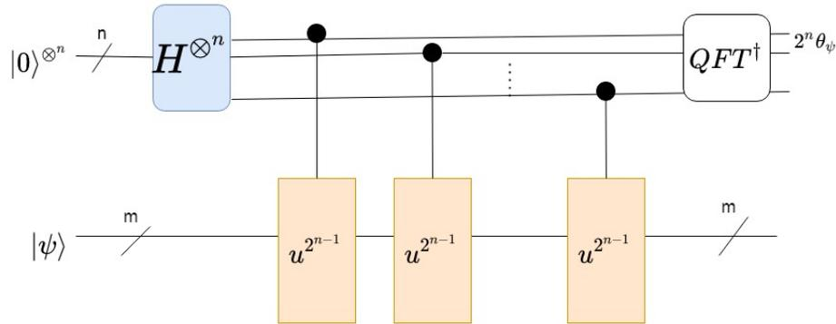
Figure 19: Quantum Phase Estimation
