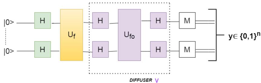
**Figure 11:** Grovers Algorithm Circuit
