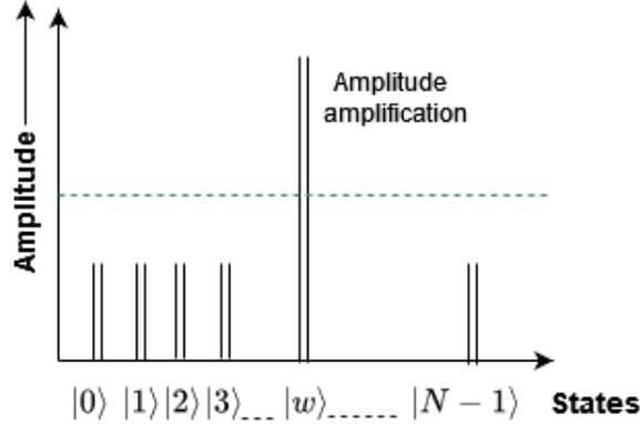
**Figure 15:** amplification about average amplitude
