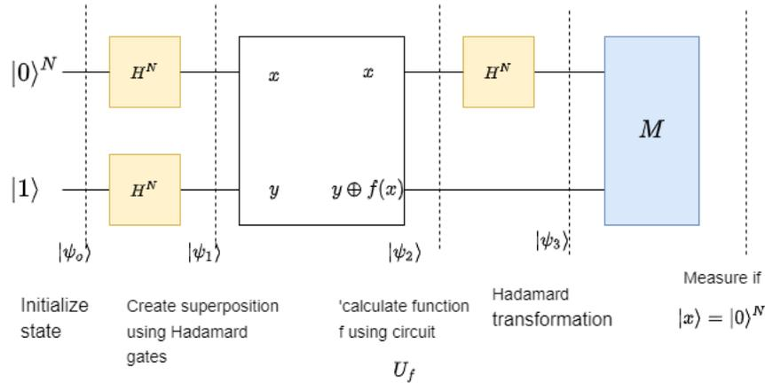
**Figure 10:** Deutsch Jozsa circuit
