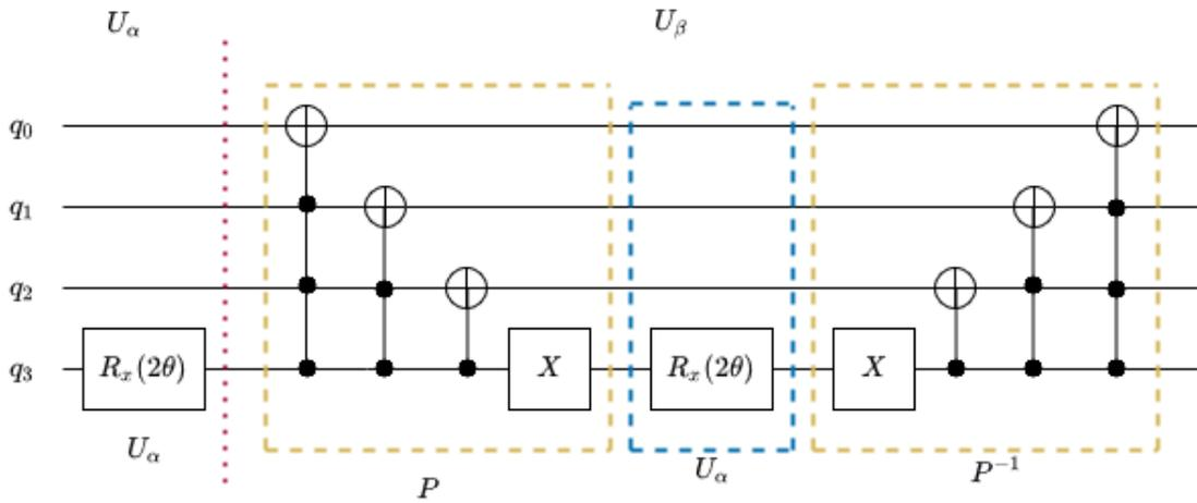
**Figure 33:** One walk step of SQW in 1D lattice using 4 qubits
