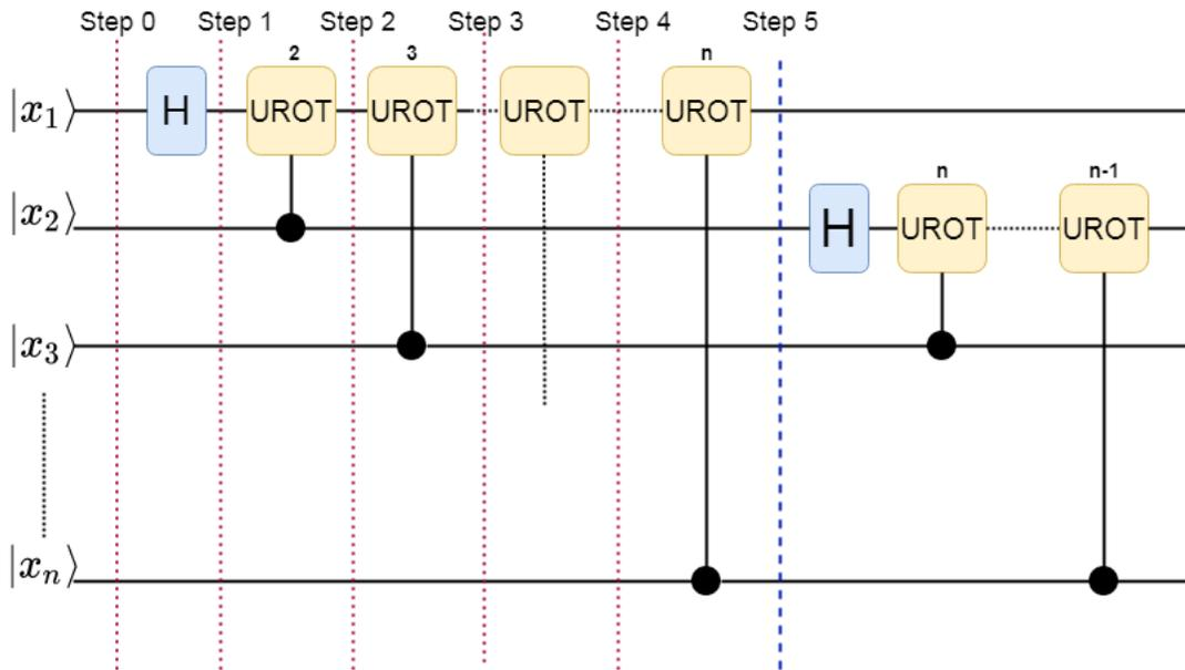
Figure 17: Quantum Fourier Transform
